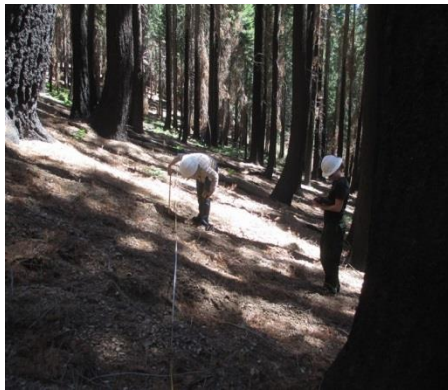
Transect data collection measuring depth and width of riling.
