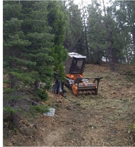
Figure 5b: Example of a front-mounted masticator.
