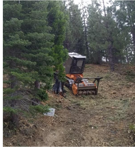
Figure 5b: Example of a front-mounted masticator.
