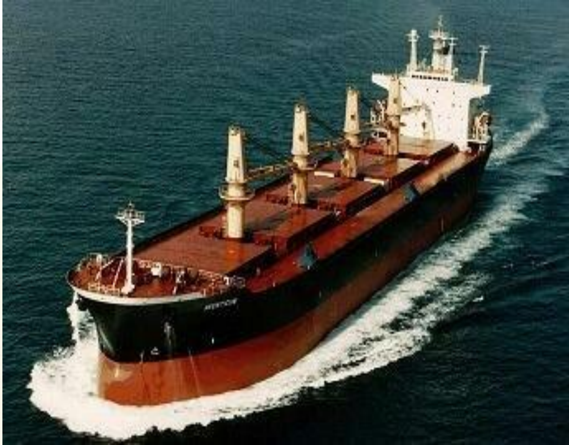
Handymax Bulk Carrier 45-50,000 Tonnes
